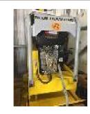
PLATE COMPACTOR, BLUE DIAMOND MOD: BDM-350 DOM: 2015 323kg FORCE, DIESEL, ELECTRIC START
