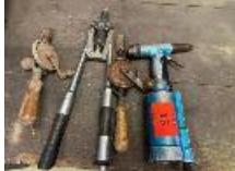
AIR OP RIVET GUN, LONG HANDLE RIVET GUN & 2 x HAND DRILLS                                                                     |      |
